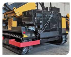
**NEW POWER PACKS** New Stage 5 / Tier 4 final compliant engines, watercooled and equipped with a diesel particulate filter
